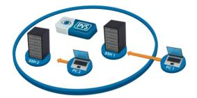
In the image shown above, the PVS is configured to monitor traffic for an enclave. It observes PC1 log into SSH1 via secure shell across the boundary as well as PC2 log into SSH2 within the enclave. The PVS has been configured with the network ranges of the enclave and PC1 has an IP address that is not part of that range. The PVS would report on any SSH vulnerabilities found on SSH1 or SSH2 but it would also tag the vulnerabilities on SSH1 as being externally facing.
